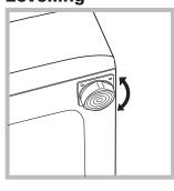
Your machine may make a considerable amount of noise if the two front feet have not been adjusted correctly.
